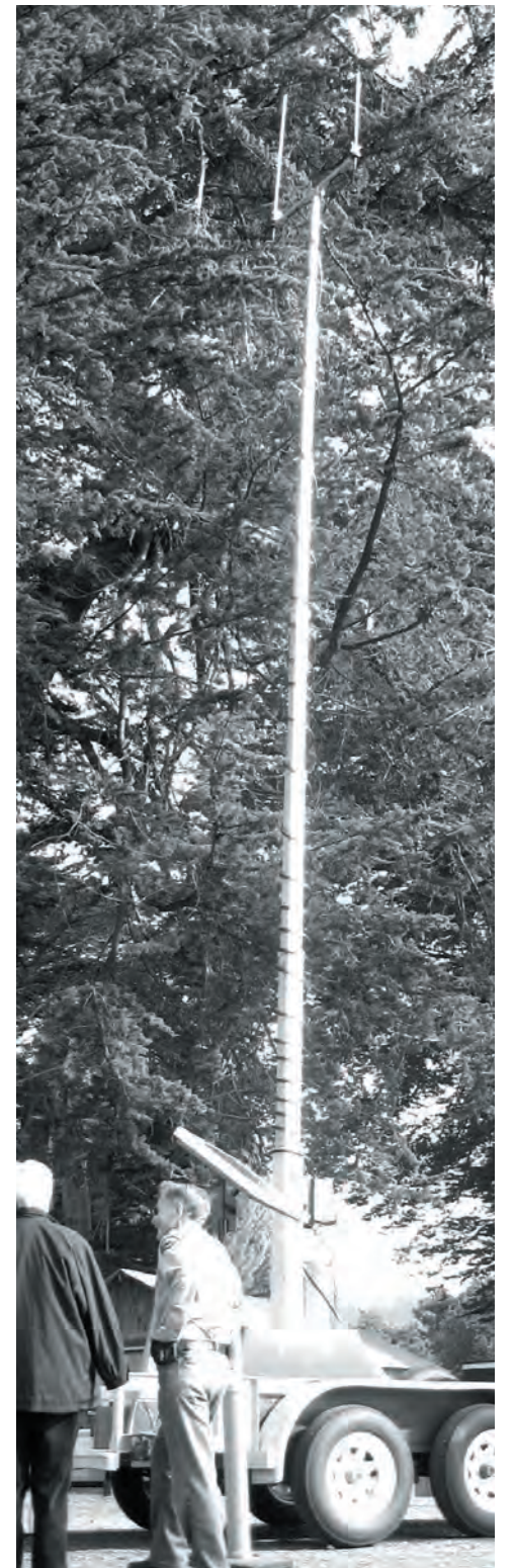
Emergency communications trailer with a solar powered radio repeater antenna.
